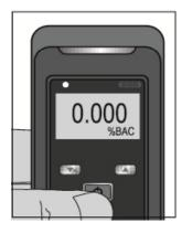
In NORMAL MODE operation a 3 decimal place result will appear on the display and remain for 15 seconds. eg. 0.051%BAC
