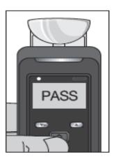
In FAST MODE operation either the word PASS or FAIL will appear on the display indicating the presence or absence of alcohol. The PASS level is 0.000 %BAC by default but can be
