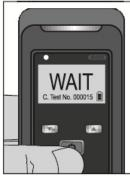
The word WAIT will appear on the display along with the number of tests performed since the last calibration.
