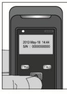
Depress the ON/OFF button for 2 seconds until the breathalyser turns on.
